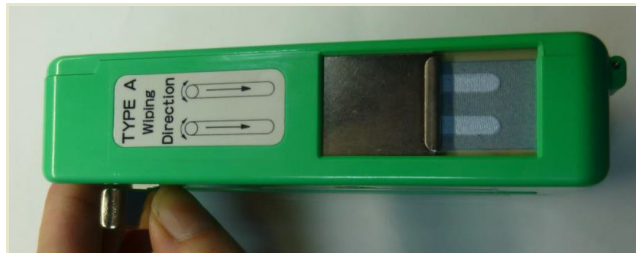
Figure 58 Example of a fiber cleaning cartridge
