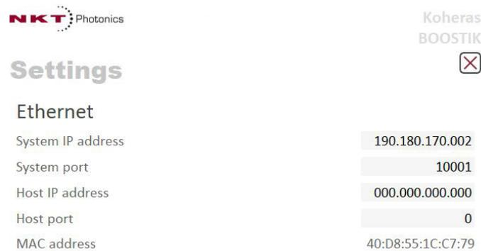
**Watchdog** The system features a watchdog for monitoring of USB or Ethernet communication. If CONTROL is disconnected from the chassis, the watchdog disables emission after the watchdog timer expires.
