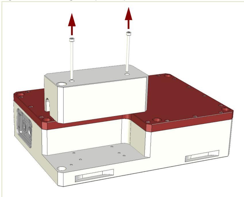
6. Mount the collimator assembly to the optics head by inserting its alignment pins into the baseplate holes, see [Figure 8](#). The lateral positioning of the collimator is defined by the two alignment pins.
