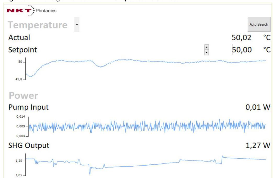
**Autosearch button** – automatically adjusts the oven temperature to the optimum.
