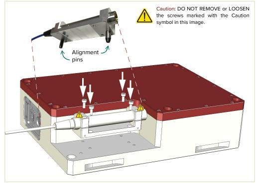
*Figure 8* Installing the collimator assembly
