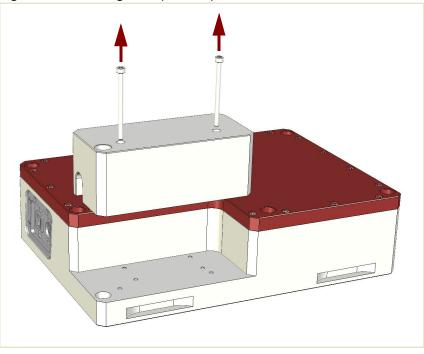
Figure 7 Removing the optical input cover
