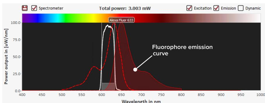
**Dynamic** When this function's *Dynamic* box is checked, you can simulate the fluorescence emission for various CHROMATUNE emission settings. The function works by dynamically modifying the fluorophore emission plots for the set wavelength, bandwidth and power as they are changed.
