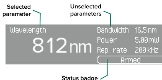
**Emission parameters** The emission parameters displayed are described in Table 16.
