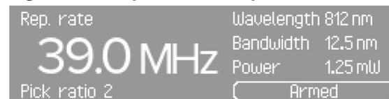
3. Use the + and – buttons to increase or decrease the Repetition rate. Conversely, the + button decreases the pick ratio and the – button increases it.
