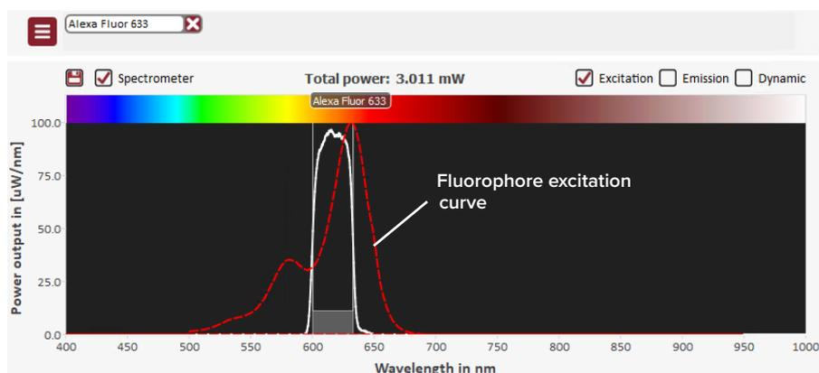
**Emission** Along with the fluorophore excitation curve, you can plot the emission data curves from any added fluorophores by checking the Emission box in the upper right. **Figure 59** shows the Excitation and Emission boxes checked and note the emission data is distinguished from the excitation data in that it is tinted underneath its curve.
