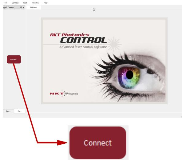
5 CONTROL automatically scans for any connect lasers and accessories available on both COM and configured Ethernet ports.
