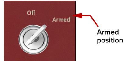
**NOTE:** The connected interlock circuit must also be closed i.e. door closed for emission to be enabled.
