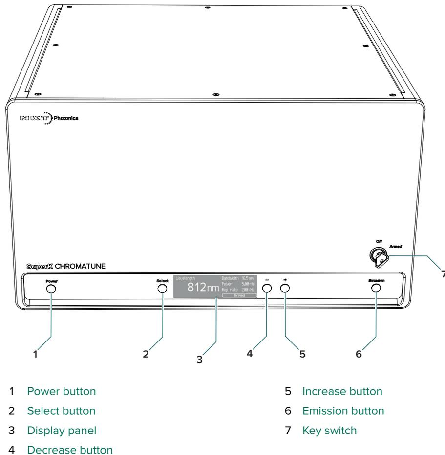
**Power button** Press this button to turn all system modules ON or OFF. The power button must be pressed for approximately 1 to 2 seconds to turn ON the system.
