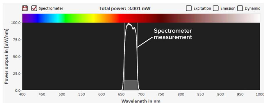
**Excitation** When using the fluorophore options of the CHROMATUNE, you can plot the excitation curve of any loaded fluorophores added to the view – see “Fluorophore control group” on page 95. To plot the fluorophore curves, check the *Excitation* box in the upper right of the view as shown in Figure 58.
