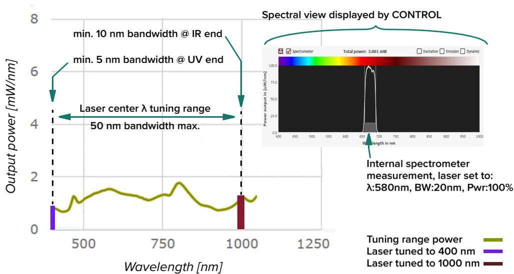
**i** **NOTE:** The laser emission is limited to the 400 – 1000nm range. If the selected emission band extends outside this range, this will in practice be truncated. For example, tuning to a center wavelength at 400 nm with a bandwidth set to 20 nm you would expect 390 to 410 nm lower and upper bandwidth limits. However, CHROMATUNE emission is limited to a minimum 400 nm wavelength, thus for this setting the bandwidth is from 400 to 410 nm.
