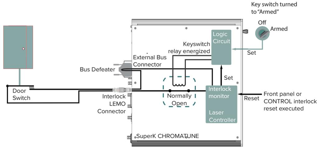
Figure 12 shows the door switch in the open position. This opens the interlock loop which the interlock monitor detects and the controller immediately sends a shutdown signal to the laser (the laser’s pump). In addition, the controller sends a reset to the logic circuit. The reset causes the logic circuit to de-energize the keyswitch and the relay opens.
