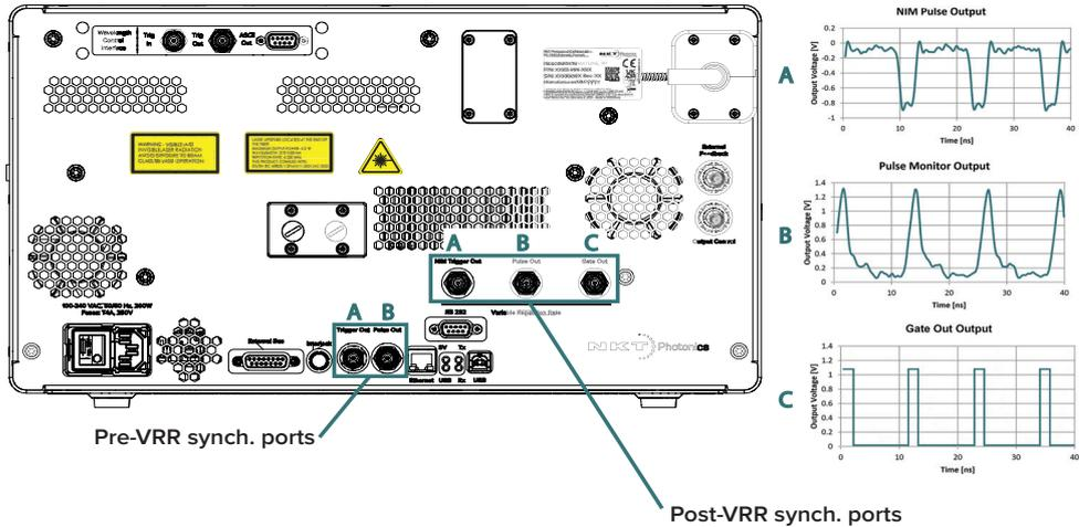
**Example synchronization circuit** As an example, the pre or post-NIM pulse signal could be used to synchronize the emission with a subject under study. A general diagram of a synchronization circuit is shown in Figure 19.
