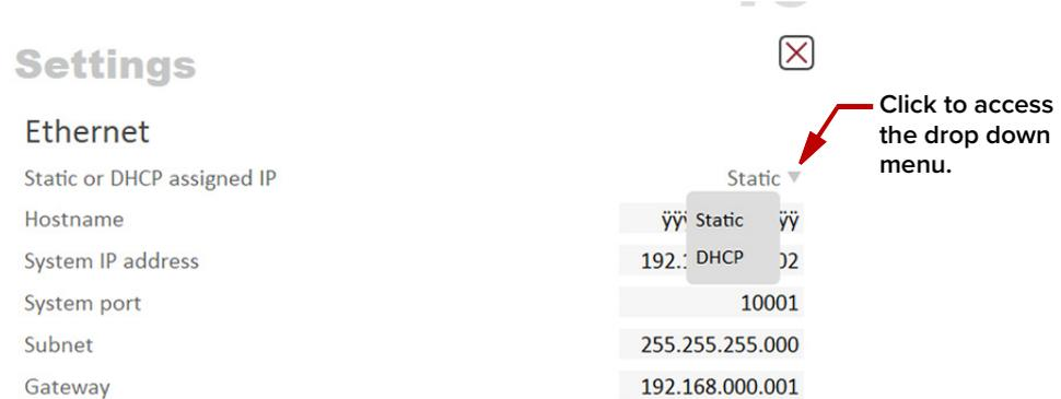
**Static network settings** **Figure 45 Ethernet (network) static settings**
