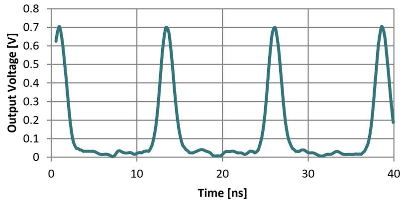
**Post-VRR ports** These interfaces provide synchronization signals that represent the pulse output after the optional VRR module.
