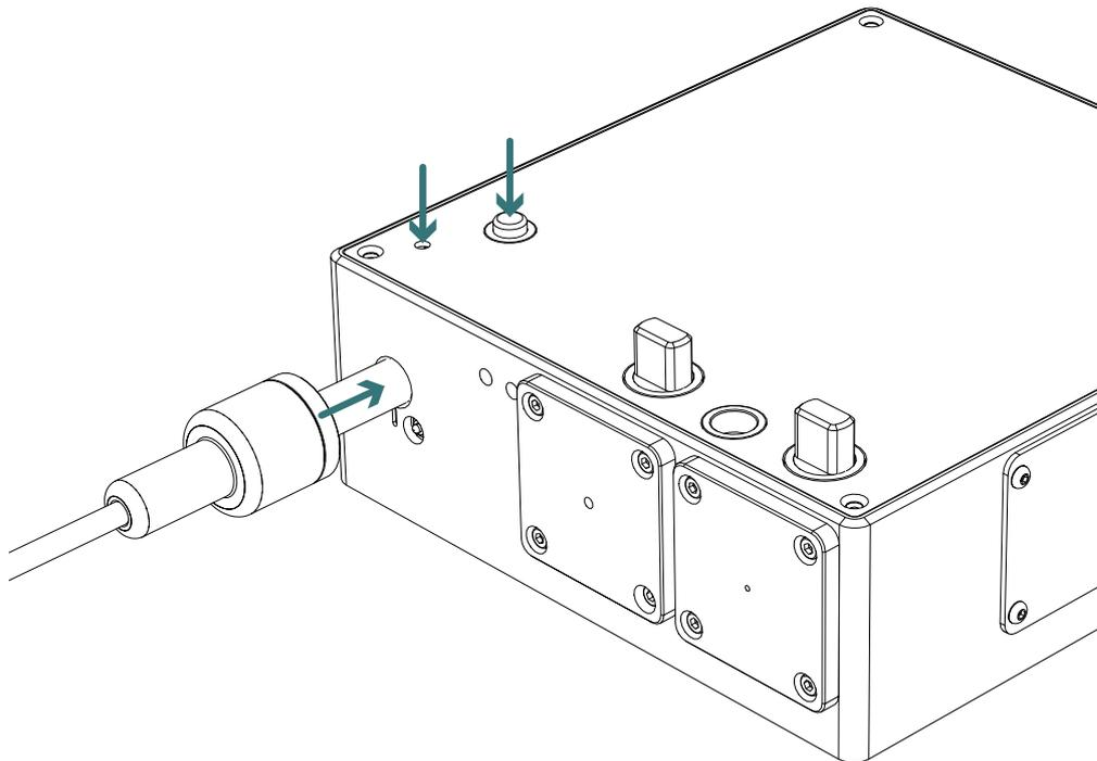
**Figure 14 Inserting a collimator into a holder**
