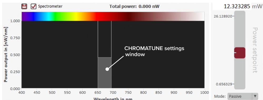
**Spectrometer** Checking the spectrometer box option turns on a spectrometer measurement function. The emission measurement is then displayed as a white line in the spectrum view as can be seen in the Figure 57.
