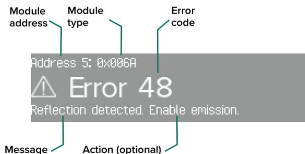
**Error identification** All errors are listed in [Table 27 on page 133 of Appendix E](#). An error is identified by its module address and the error code:
