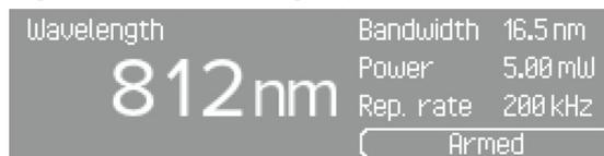
3. Use the + and – buttons to increase or decrease the set center wavelength value in increments of 1 nm.
