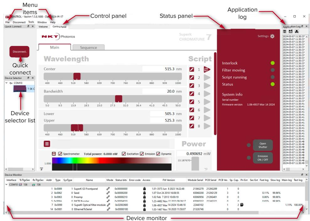
**Relocating panels** You can drag the different panels of CONTROL to any location within the main interface or into a separate floating panel. [Procedure 17](#) describes how to relocate a panel within the main window:
