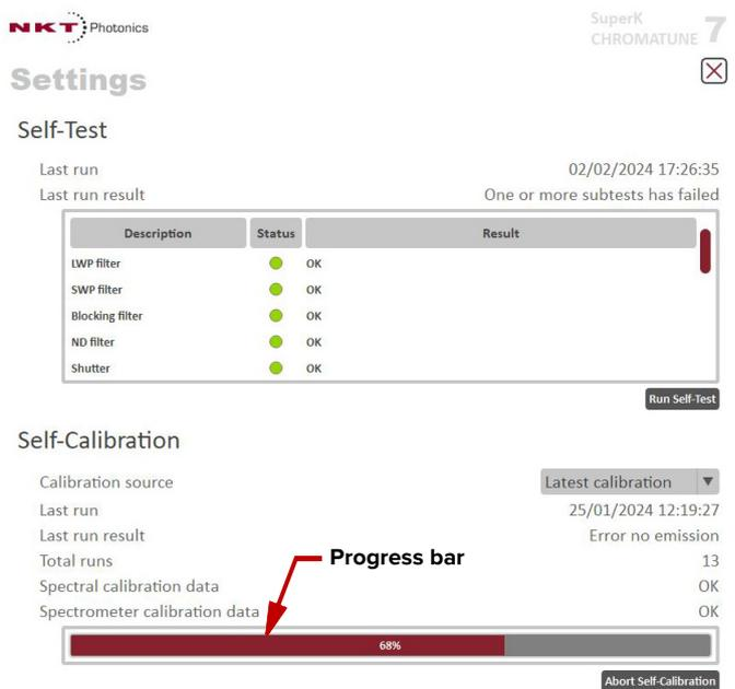
The screenshot shows the 'Settings' page during the self-calibration process. The 'Self-Calibration' section shows a progress bar at 68% with a red arrow pointing to it. The 'Run Self-Calibration' button is now labeled 'Abort Self-Calibration'.
