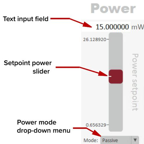
**Power mode** The method the CHROMATUNE uses to determine and control the output power can be changed by selecting one of 5 modes from the power mode drop-down menu shown in [Figure 65](#). The selectable modes are as follows:
