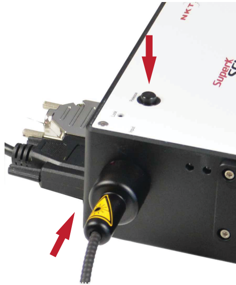
Figure 49 Collimator Installed in a Holder Receptacle
