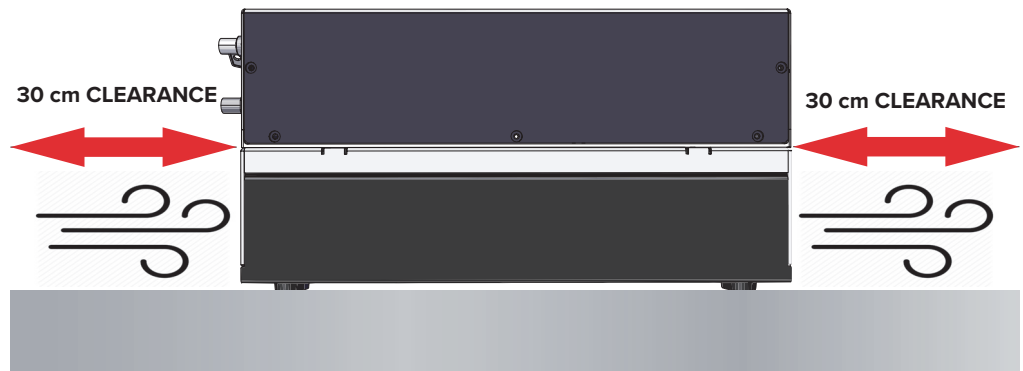
Figure 12 Air cooled SuperK EVO – airflow clearance
