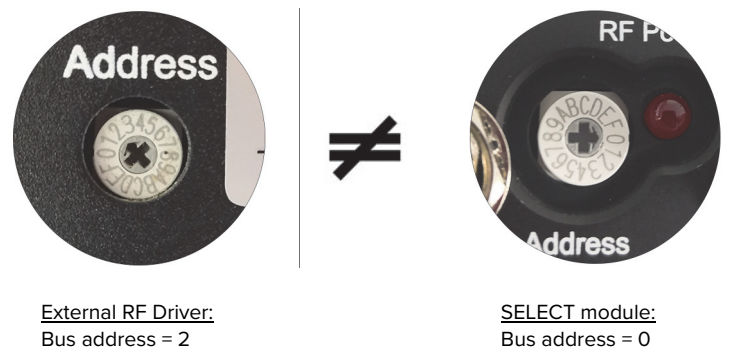
Figure 19 Setting External bus addresses - single ERD system
